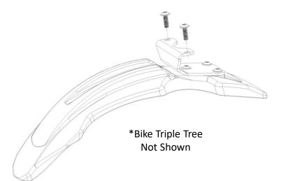
step 2. Slip the bracket over the lower triple tree on the bike. Start threading the remaining two bolts through the bracket and into the threaded holes in the triple tree. When both bolts are started straight, check the alignment of everything and then tighten them up!
