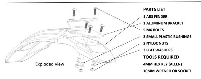
**STEP 1.** Attach the fender to the bracket using 3 bolts from the top of the bracket. Use the plastic bushings, the washers, and the nuts from the bottom side. Make sure the fender is aligned well before tightening the three bolts. Make sure the bushings are staying in the oversized holes in the fender!
