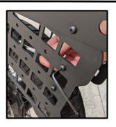
7. Once all hardware is started, tighten all bolts and nuts with a 3mm allen key and 8mm wrench. Don't over-do it. These nyloc nuts will stay snug for many miles to come.
