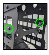
5. Next, you'll need the support/ license plate bracket. Orient the bracket at the rear of the MOLLE plates with the mouning tabs facing towards the front of the bike. Align the bracket so the holes match-up with the uppermost and rearmost holes in the MOLLE plates.
