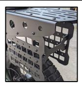
6. Place bolts with washers through each of the 4 holes. Washers and nuts are then threaded onto the bolts from the inside. Ensure all the hardware is started but not tight yet.
