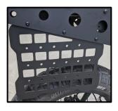
3. Insert a bolt and washer through the brace and the MOLLE Plate. Place a washer and a nut on the back side and thread into place. DO NOT TIGHTEN YET. We'll get to that later I promise;)
