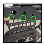
2. Align a MOLLE plate with the mounting holes along the lower edge of the R-S Back Rack side brace.
