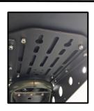
8. Place washers and nuts onto the 4 bolts from the underside of the rack and tighten with the allen key and wrench. Double check that all hardware on the crate is secure.
