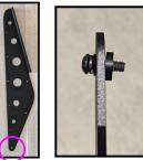
2. Put one Bolt/Washer stack through the hole in the Brace from the flat side of that part. Starting with the front hole circled in the image above. Next, slip 1 of the plastic spacers onto the bolt as shown above and start threading it into the hole shown in the next image. Repeat EXACTLY for the other hole. DO NOT TIGHTEN YET. Please;) Now repeat on the other side!
