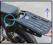
7. Finally time to tighten! Lift up on the back of the rack to remove any "play". While you're doing that, snug the bolts going into the bike frame. After that, snug down the strut bolts. Double check that none
