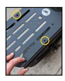
4. With the Top Plate on the Braces and aligned with the 6 holes, slip a bolt with a flat washer into each of the 6 holes. From the underside put a flat washer and a nut onto each of the 6 screws. Once all the nuts are started, begin tightening all of these 6 bolts. Looks good but we're not done!
