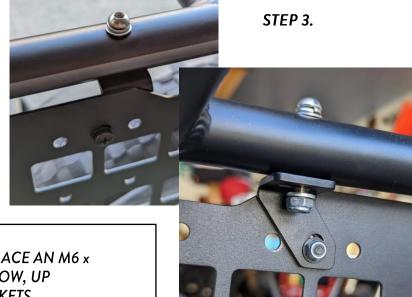
STEP 3A. IF YOU ARE USING A REAR SEAT, PLACE AN M6 x 45MM BOLT AND AN M6 WASHER FROM BELOW, UP THROUGH THE SLOTS IN THE ANGLED BRACKETS, THROUGH THE HOLES IN THE BIKE FRAME AND INTO THE BUILT-IN NUTS IN THE SEAT. AFTER TIGHTENING THESE BOLTS, RETURN TO ALL THE OTHER HARDWARE FROM THE PREVIOUS STEPS TO TIGHTEN EACH OF THEM.
