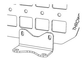
**STEP 2.** Place the assembly onto your Rad Runner bike and align with the threaded holes on the frame. Using a total of 4 M5 bolts with a lock washer and a flat washer on each bolt, thread the bolts through the L-Brackets and into the threaded holes on the frame. Start all the bolts before tightening any of them. Once all the bolts are started, tighten securely. Next, adjust the position of the MOLLE Panel and tighten the hardware from Step 1.
