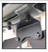
6. Starting at the top, get 2 bolt and washer stacks started into the threaded holes on the bike. You aren't going to tighten them until you have all 8 bolts started around the frame. Go ahead and snug all the bolts down. Don't go crazy though, the threads in the bike are aluminum and you can strip them if you get all He-Man on them. Google He-man if needed.
