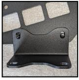
1. Place the MOLLE panel flat with the logo upwards. Grab a bracket and line it up with the attachment slots. Make sure the slots in the bracket are in the SAME orientation as they are on the panel. Push through 2 bolts (with no washers) from the back side.
