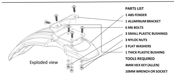
STEP 1. Attach the fender to the bracket using 3 bolts from the top of the bracket. Use the plastic bushings, the washers, and the nuts from the bottom side. Make sure the fender is aligned well before tightening the three bolts. Make sure the bushings are staying in the oversized holes in the fender!
