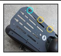
**5.** Place a bolt with a flat washer through each of the three holes along the edge.
