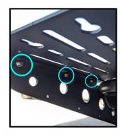
7. From the underside put a flat washer and a nut onto each of the 6 screws. Once all the nuts are started, begin tightening ALL the hardware. Nice work, You're done!
