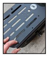
6. Flex the opposite side Brace and the Top Plate together until the 3 holes align. Slip a bolt with a flat washer into each of the three holes.
